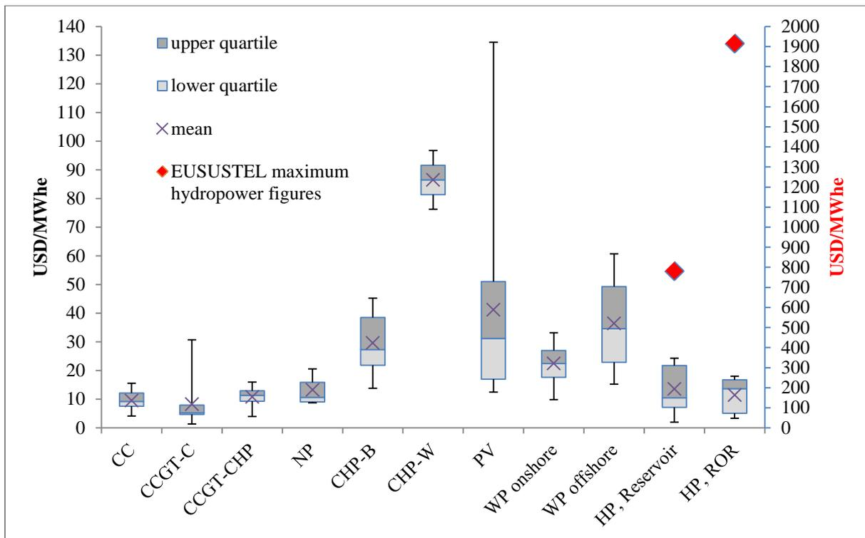
**Figure 9.** Presented O&M costs in the reviewed studies (i.e. [4], [5], [7], [8], [10-15], and [18]). Note that two y-axis scales are used, where the second rightmost one is used to visualize the stated maximum EUSUSTEL hydropower figures.
